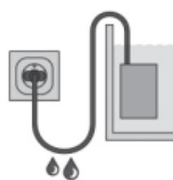
This prevents any water running along the cable to the mains socket, which would result in a short-circuit.
